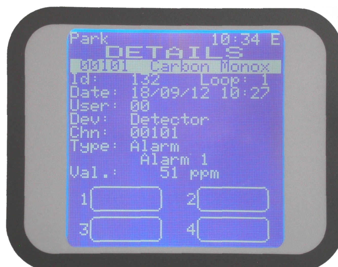
Figure 22 ALARM details screen.
